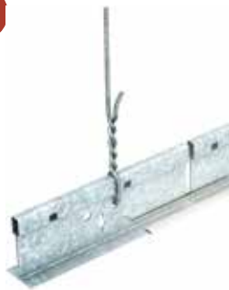
Rondo 120 soft galvanised wire secured with three tight 360° turns
