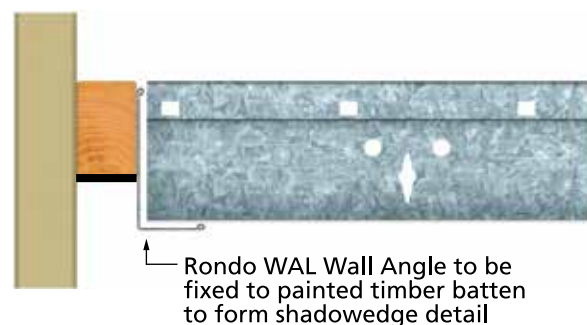
■ LONG LEG WALL ANGLE TYPICAL APPLICATION
