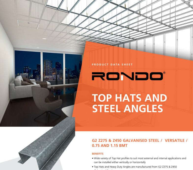
Rondo Top Hats can be used internally or externally and on vertical fascias and soffits. They are often used where there is a higher wind loading or where heavy duty sheeting is to be installed.
